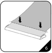
6. Attach Velcro strips to the bottom of the back of banner.
