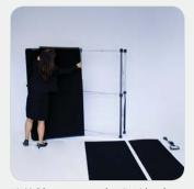
12. Hold a center panel on its side edges about 1/3 of the way down from the top. Lift section and guide notches over the panel pegs on the top hubs. Slowly release the panel, allowing it to roll down the channel bars. Repeat for all center panels aligning them as you go.
