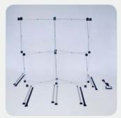
4. Set up the channel bars to the frame. 4 black channel bars go on the 4 outer lower positions (There s velcro which holds down the lower corner of the endcaps) and rest of channel bars go on the middle lower positions and all top positions.
