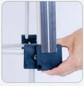
Slide the bottom of the channel bar from right to left onto the metal peg. Continue with the middle and lower channel bars.
